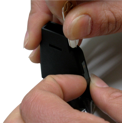
BATTERY TOOL to unlock the battery tray
