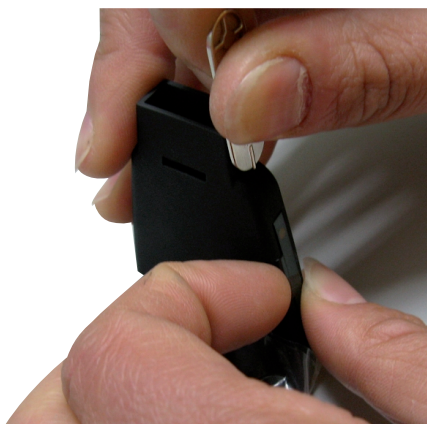
BATTERY TOOL to unlock the battery
